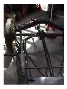
We obtained drawings of the tail pipe from the Ford Archives and also found a fellow with an original tail pipe(rusty), we used these two items to create the reproduction tail pipe. It is almost identical to the sample we had and after some minor adjustments, it will fit any Model A, not just the Station Wagon and Delivery vans.
