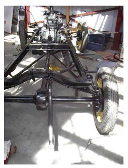
Photo at left is looking from the rear. Note the pipe crosses over and is supported at the frame, just like the stock muffler. The tail pipe is clamped to the rear of the muffler. We provide a short stub on the back of the muffler for this connection.
